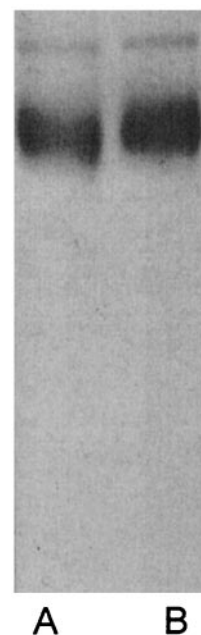
FIG. 1. Electrophoretogram of ferritin: (A) isolated ^{59}\text{Fe} -labelled rat ferritin; (B) standard rat ferritin purchased from Sigma Chemical Co.
